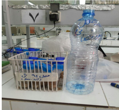
Figure 2- Preparation of the samples for testing (samples after grinding combined with the solvent).
