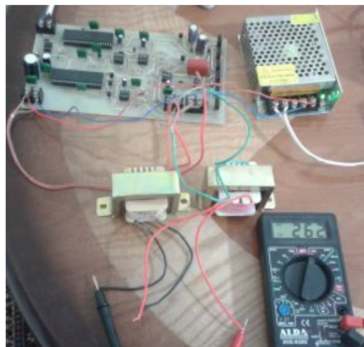
Fig.9. A photograph of the proposed grid-tied inverter
