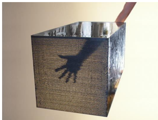
Figure 3. A Litracon concrete (Source: http://openarchitecturenetwork.org )
